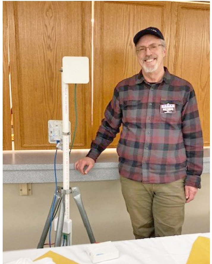
Ben Bowers, KE3KQ, describes his recent efforts to establish a network RF communication link in the field using a battery-powered portable two-node system.
