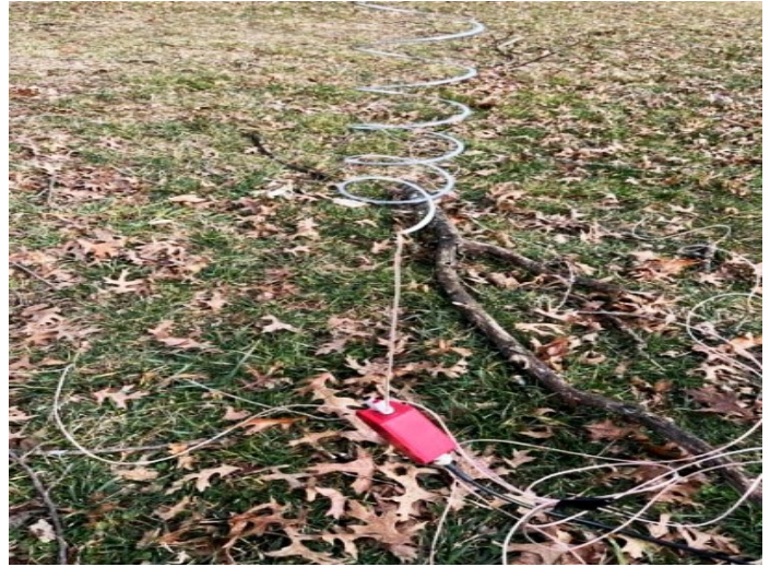
The Slinky antenna was terminated with an LDG 9:1 unun.
