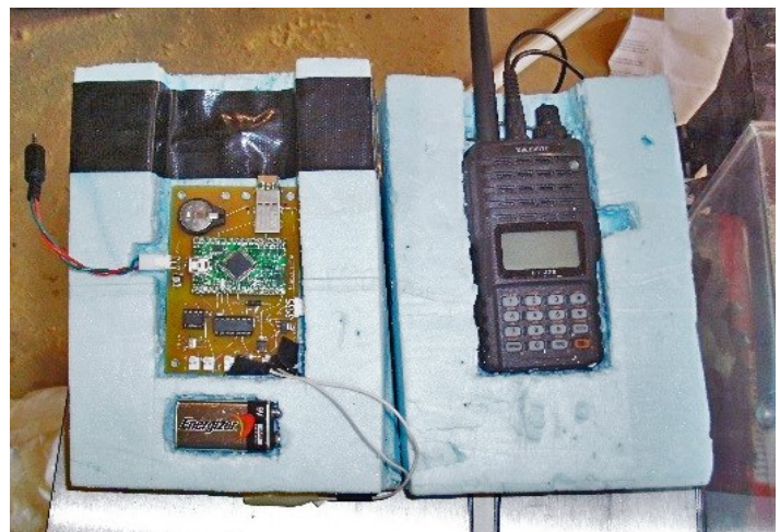
AC9L's kite transceiver payload equipped to send APRS data.
